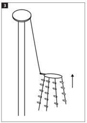
3. Fasten the product to the ground around flagpole. Make sure all the parts of the product are evenly spaced to each other and the flagpole. Roll up surplus string light on the bobbins.
