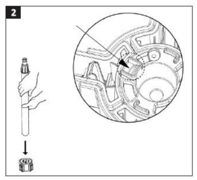
2. Fit the 4 parts of the foot on the connecter and check that they are firmly in place. FIG. 3 & FIG. 4
