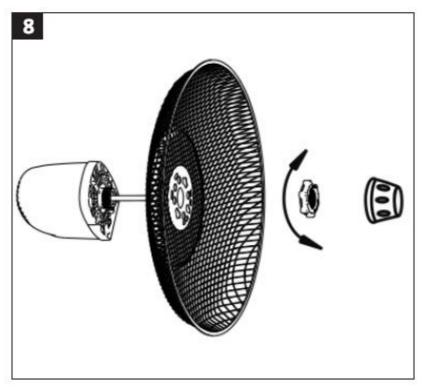
2. Put the fan blade on the axle and check that the pin on the blade axle engages in the slot in the fan blade. Turn the hub nut anticlockwise to lock to lock the fan blade. **FIG. 9**
