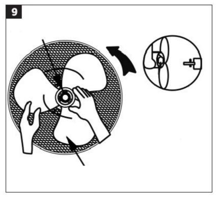
3. Put the front and back grille together with the grille clamp and tighten the lock screw and nut for the grille.
