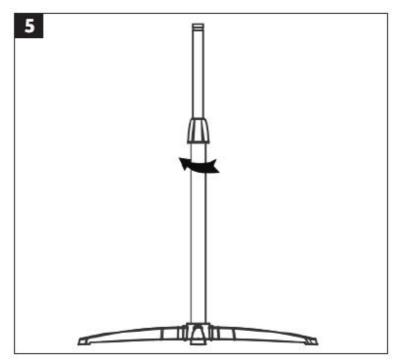
4. Release the height adjustment ring on the column tube and adjust to the required height. Tighten the height adjustment ring. **FIG. 6**
