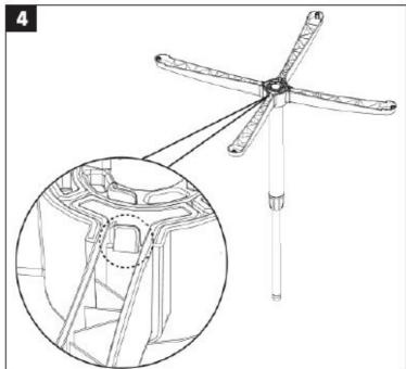
3. Put the column tube in the connector from above and check that it locks in place look from underneath through the hole in the connector. **FIG.5**
