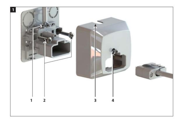
Releasing the casing Release the casing as shown.
