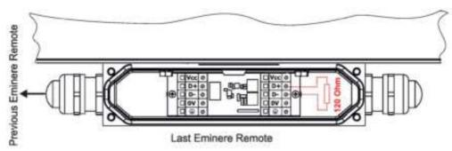
Number of connected Emineres to one LED output of the E-box Remote depends on the type of Eminere Remote and cable length.
