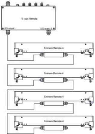
**NOTE:** Each line of Emineres Remote connected to the LED output of the E-box Remote has to be terminated at the last fixture.
