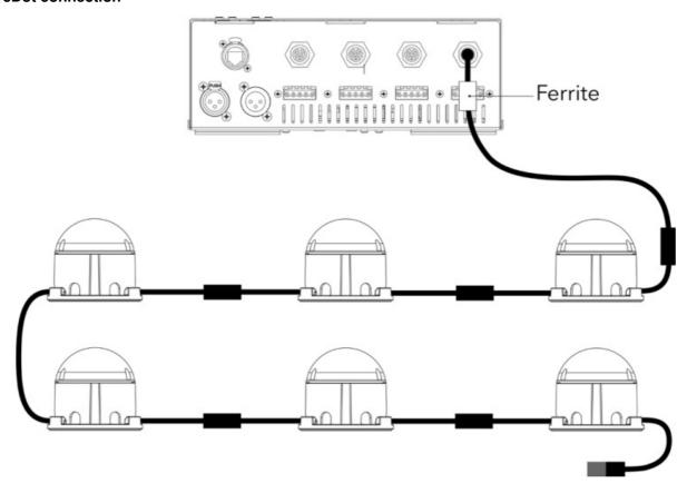
ArcDot line may be done with in/out connection or by using T-connectors (1 ArcDot can be connected to T-connector). Max. number of ArcDots per output is 35. Max. cable length of 1 LED output is 65m at 35 ArcDots and 100m at 25 ArcDots per LED output.
