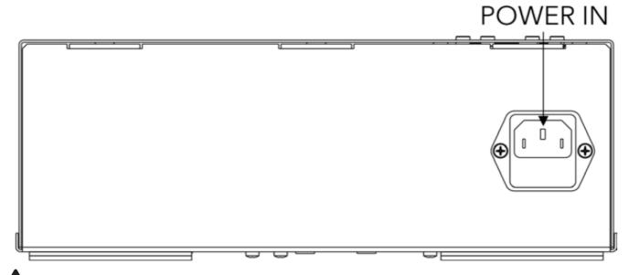
Maximum length between the ArcPixel Power and the last fuxtures must not exceed 100 meters. Do not connect or disconnect LED modules when ArcPixel Power is under voltage. If the line of fixtures is disconnected,
