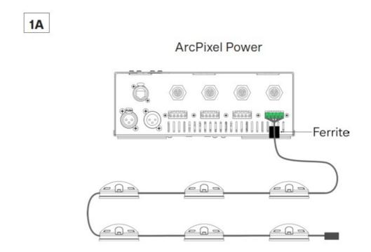
Install terminal blocks on cable and connect it to the LED outputs of the ArcPixel Power.
