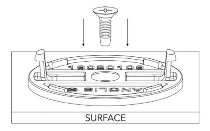
Take care not to over tighten the fastener to avoid damaging the mounting adapter.
