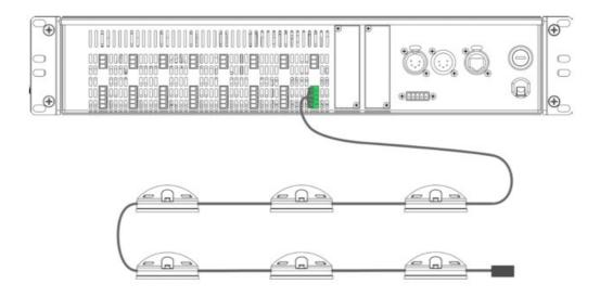
Install terminal blocks on cable and connect it to the LED outputs of the ArcPower Unit Pixel.
