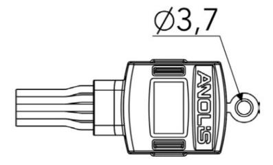
The hole in the housing of the termination box serves for screwing to the mounting surface.
