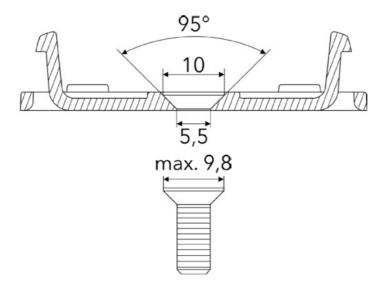
Length, diameter and type of screw depends on conditions of installation. The head of the screw should not be sticking out of the mount adapter. Otherwise, the ArcPix II may not seat properly in the mounting adapter.
