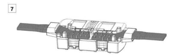
The cable cores are pressed by the cover and pushed to the
