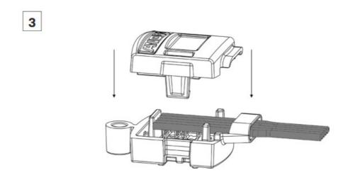
Put the cover on the base and press both parts together until both plastic catches snap into slots in the base of the termination box. For pressing use suitable plier with flat jaws if necessary.
