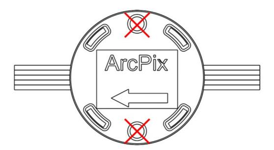
Every ArcPix II has an identification label with arrow on the bottom side. When you do your installation, keep the same orientation of the ArcPix II lines to ensure the same light characteristic of each line.
