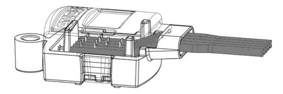
The cable cores are pressed by the cover and pushed to the contacts in base.
