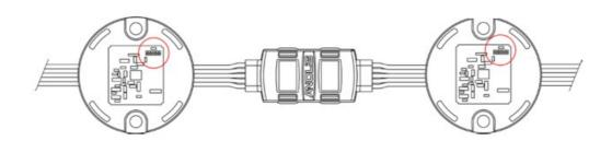
Check the correct position orientation of the new ArcPix II before connecting it into connection boxes.
