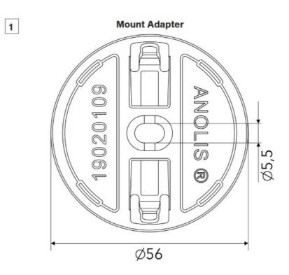
Drill hole to the mounting surface according to mount adapter holes spacing.
