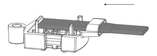
Separate wire cores from isolation at length cca 40 mm on the end of the 5-wire flat cable. Insert the 5-wire flat cable through the bushing into the base of the termination box until it touches the partition in the termination box and align the cores into cutting edges.
