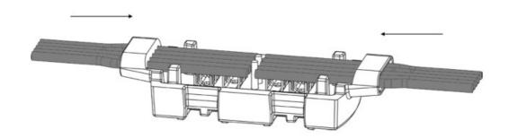
Separate cores in length 40 mm on the end of 5-wire flat cable. Insert cable trought the bushing into base of the connection box until it touches the partition in the connection box and align the cores into cutting edges.
