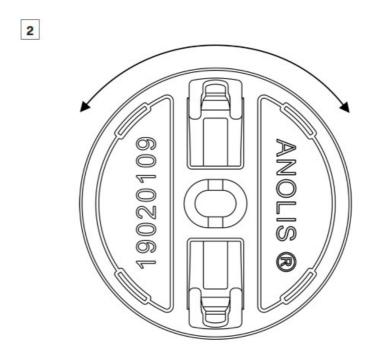
Prepare the correct mounting position of the adapter, making sure that all of them are oriented in the same direction.
