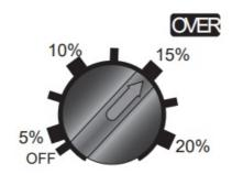
Set the desired value for over voltage. This function can be turn off by turning the knob to off position.
