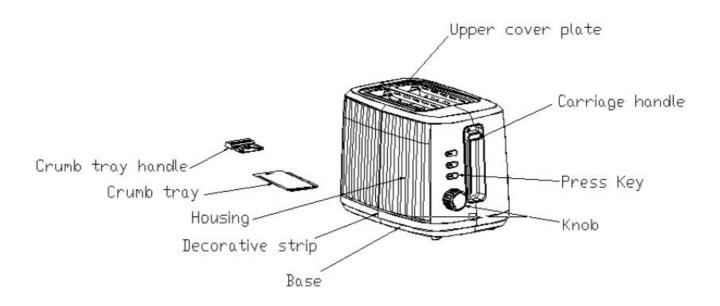
Du ring manufacture, residue or oil may remain in the toaster or heating element which is likely to emit an odo u r when used for the first use. This is normal and should disappear after a few minutes of use. When the toaster is used for the first time it is suggested to operate according to the below steps, except without bread. Then let the toaster cool down and begin toasting the first slice.
