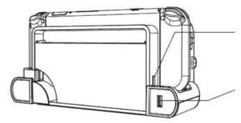
The USB female port on the original dock can be connected to an external wired controller
