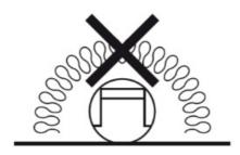
The power supply that can be used where normally flammable materials.including building insulation, are or may be present, but cannot be abutted against any material and cannot be covered in normal. Minimum clearance distance from the top and sides of the control gear to normally flammable building element is 75mm; as shown in below picture, A=B=C=Min.75mm.
