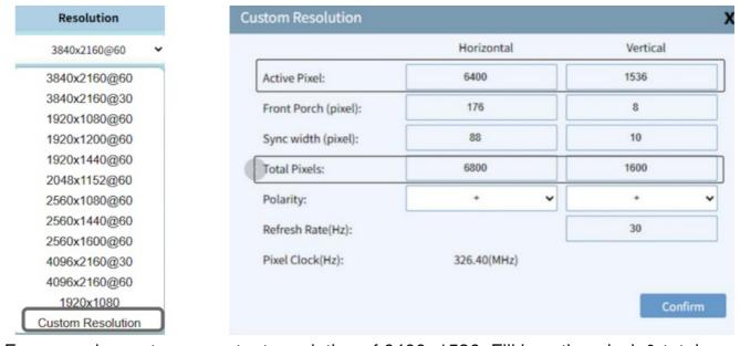
For example, custom an output resolution of 6400×1536. Fill in active pixels& total pixels.
