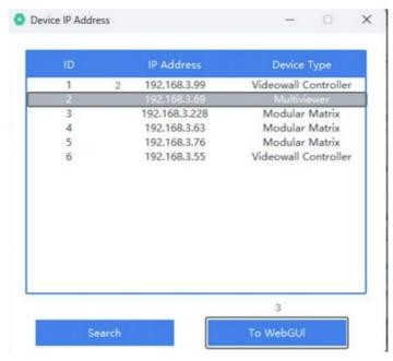
• **3rd Step:** Manually set the control computer IP address, which needs to be in the same network segment as the Multiviewer.
