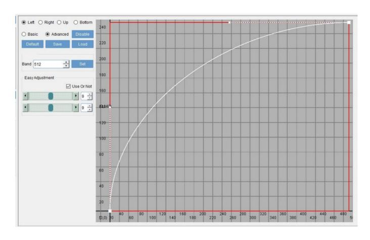
**Advanced adjustment method:** If above methods cannot meet the edge blending feathering effect, you can right-click anywhere on the white slash and choose to add an auxiliary point (At this time, you need to unselect the item "Use or not". As shown below:
