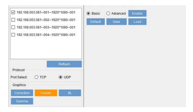
• As shown above: Select the output port and click the menu "Fusion". Then select the image edge blending direction in the upper right corner. Finally click the menu "Enable" to open the adjustment interface as shown below:
