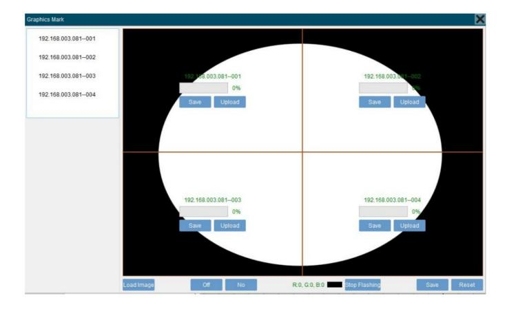
**Load image:** Select and load a image. The image resolution must be the same or exceed the input resolution. There are black and white. The black area defaults to the area that needs to be masked and not to be displayed.
