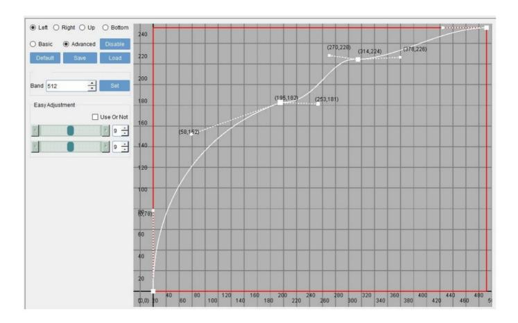
Select the added point. When the point turns red, you can drag it up and down to make it an upward parabola. At the same time, you can use the auxiliary points on both sides for uniform feathering. As shown in the below, multiple auxiliary points can be added. You can adjust it according to display effect of different projectors.
