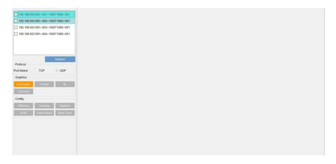
Double-click Transform\_Fusion.exe or Edge\_Blending.exe to enter the main interface as shown above. The information displayed in the upper left corner is the device IP address, output port, output resolution and the device machine code.
