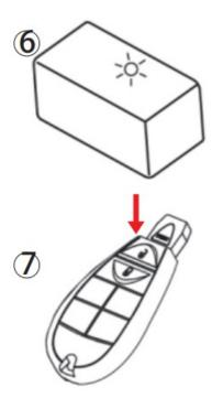
After 2~20 seconds (it depends on your vehicle), you will hear a single beep sound from the programmer. Then turn off the ignition and remove the original key from the ignition.
