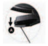
2. Pull the stylus forward and push downward to remove it from the cartridge.
