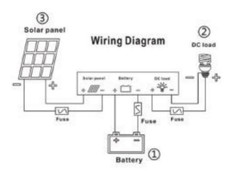
**Note:** Reversed battery polarity will not damage the controller, but you may bear security risks on your load equipment.
