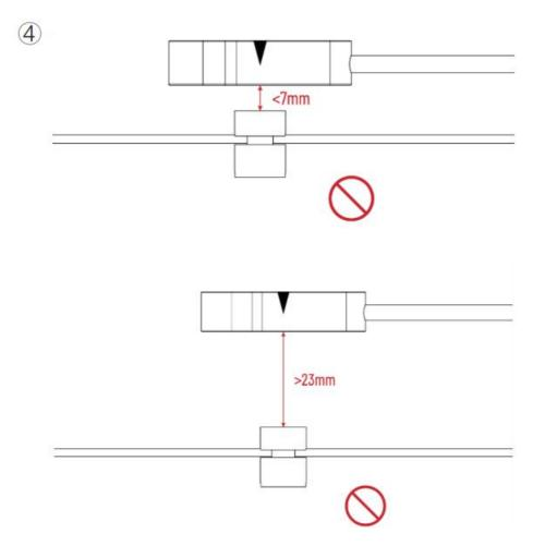
5. Adjust the speed measuring magnet to meet the above inspection requirements.
