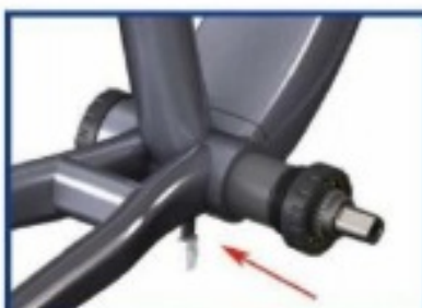
Step 2: Insert the torque sensor assembly through the left side of the bottom bracket, and pull its wire out of the lower hole of the bottom bracket.
