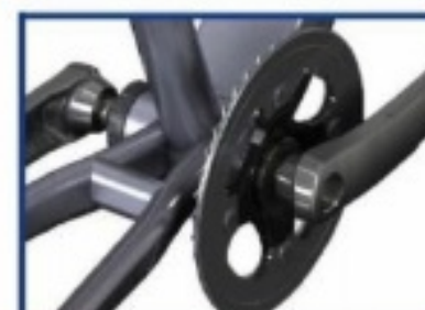
Step 6: Install the crank. Thus, the torque sensor installation is completed.
