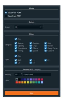
• Load a preset at any time on Program or Preview by clicking on the preset number or using drag and drop the preset into the Program or Preview windows.
