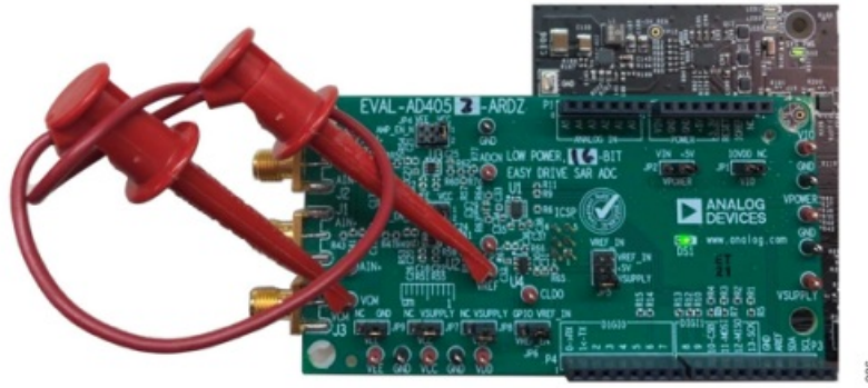
Figure 6. Biasing the EVAL-AD4052-ARDZ Inputs Without Signal Generator Hardware for Software Validation
