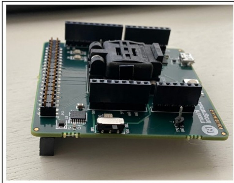
Figure 2. MAXQ1065 Socket Board with an Elevated Header Installed
