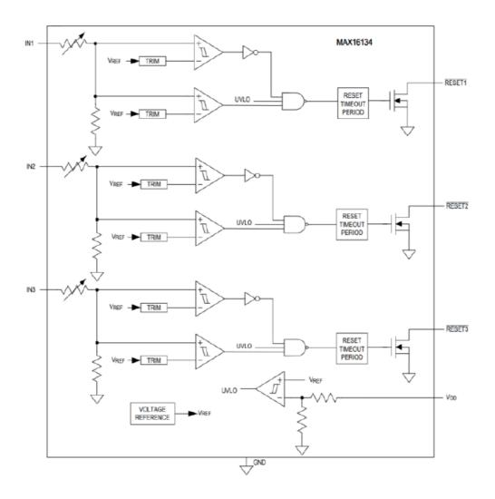
Figure 1-1 MAX16134 Block Diagram
