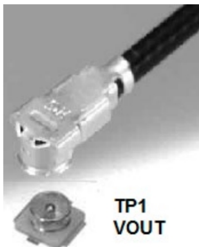
Figure 3b. Technique for Measuring Output Ripple and Step Response with a Low Inductance Connector (Not Supplied)
