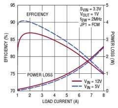
Figure 1. LT8625S Demo Circuit DC3219A Efficiency vs Load Current (Input from V<sub>IN</sub> Terminal)
