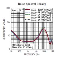
Figure 4. LT8625S Demo Circuit DC3219A Noise Spectral Density (12V Input to 1V Output, f<sub>SW</sub> = 2MHz)
