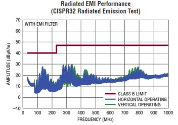
Figure 3. LT8625S Demo Circuit DC3219A EMI Performance (12V Input to 1V Output at 3A, f<sub>SW</sub> = 2MHz)
