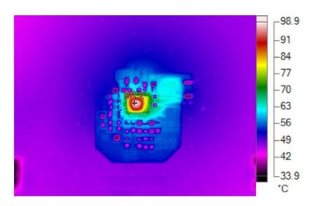
Figure 7. Thermal Performance at  $V_{IN}$  = 12V,  $f_{SW}$  = 2MHz,  $V_{OUT}$  = 1V,  $I_{LOAD}$  = 8A,  $T_A$  = 25°C
