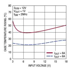
Figure 2. Temperature Rising vs V<sub>IN</sub>
