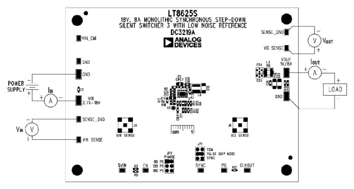
Figure 5. Proper Measurement Equipment Setup
