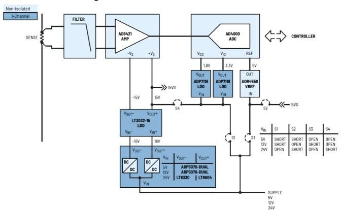
Generic Signal Chain for Current Measurement **Shunt**: Common Mode Voltage Up to 18V
