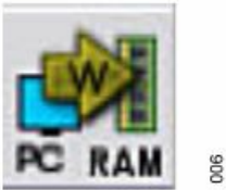
Figure 6. PC to RAM Button Transfers Data Programmed from the GUI to the LTC4286 Volatile Registers
