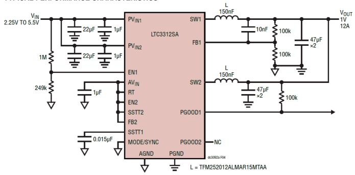
• LTC3312SA 2-Phase 2MHz 12A Buck Typical Application Schematic
