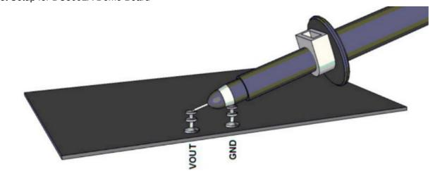
• Technique for Measuring Output Ripple and Step Response with a Scope Probe
