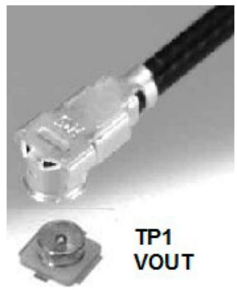
• Technique for Measuring Output Ripple and Step Response with a Low Inductance Connector (Not Supplied)
