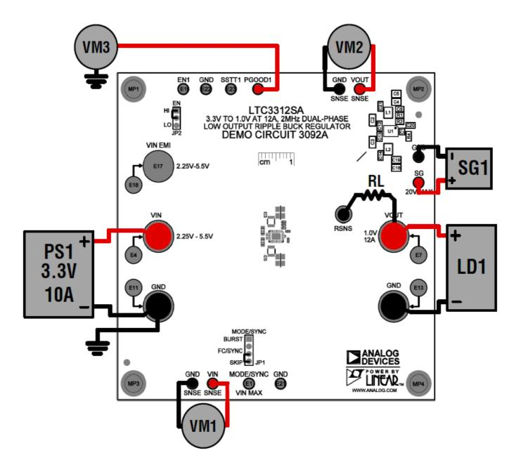
• Test Setup for DC3092A Demo Board
