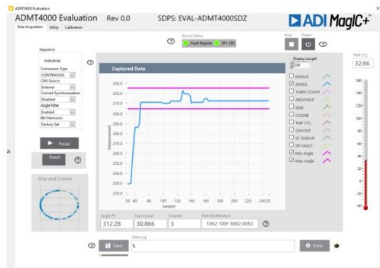
Figure 19. Captured Data Display Showing the Acquired Angle (Blue) and the Target Maximum and Minimum Angle (Magenta) for the Magnetic Reset
