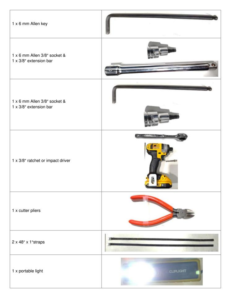
Required items when replacing actuators S-0153 or S-0204
