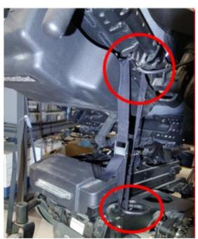
5. Completely retract (close) tilt actuator if not already done and disconnect the actuator cable. If the actuator can no longer move with power, manually screw actuator shaft to its minimum length. Using the 3/8" extension bar or the ratchet's handle as a lever, insert it into the actuator shaft hole to finish tightening it.
