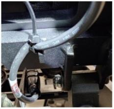
Attaching new actuator cable on the seat support for tilt systems installed after September 2020
