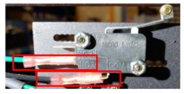
4. Move the power tilt. The drive lock-out switch should activate when the tilt reaches a 15° angle from seat pan to base.
