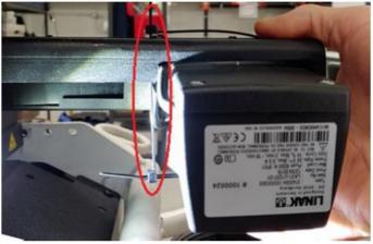
d. Cut excess tie off, flush with head, and make sure no sharp edges remain. The result should look like the images shown below.
