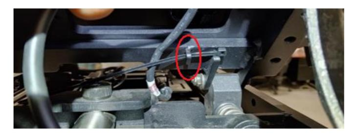
b. Loop the tie-wrap behind the cable back toward the cable fastener aligned with the first line previously drawn on the cable. Do not overtighten tie-wrap to avoid creating a crimp in the cable. Cut excess tie off, flush with head, and make sure no sharp edges remain.
