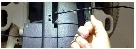
c. Join both tie-wraps together and use them to wrap around the motor compartment of the actuator to insure a stable installation of the cable. The head of the long tie-wrap must end up on the top corner of the motor compartment toward the back of the chair. The head of the medium tie-wrap must end up on the lower corner of the motor compartment toward the back of the chair.
