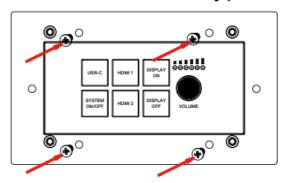
**Note:** Use the two screw holes on the left and right ends to install the EK version wall-plate TX and keypad into UK standard back boxes.
