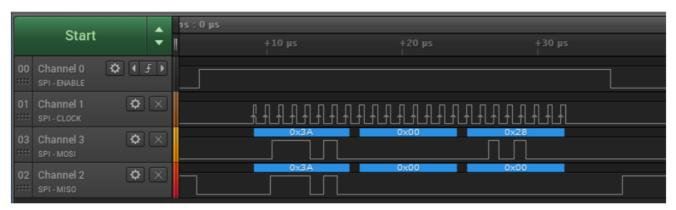
3. SET FREQ Register (Address 0x31) to 0x03 -> set fOUTDriver=125 kHz
