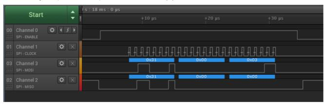
5. SET SEN0 Line to the Sensor Driver (enable SEN0 Line) (Address 0x33; Value 0x01)
