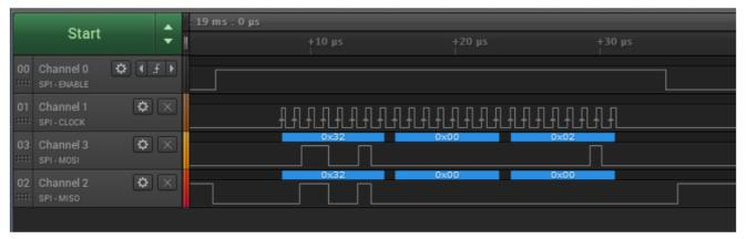
7. Start Continuous Conversation (write 0x2A into address 0x3A)
