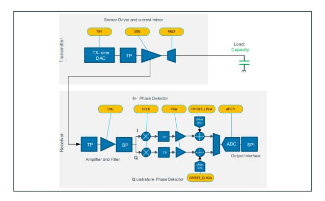
Figure 3: Configurable Parameters
