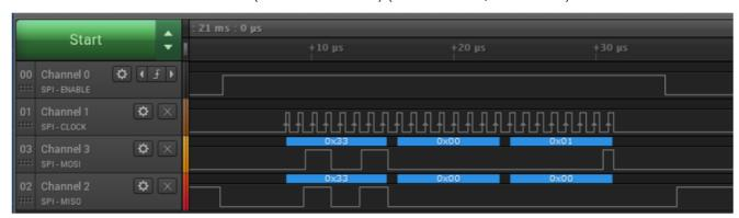
6. Reset DSP & ADC Stop (Write 0x28 into Address 0x3A)
