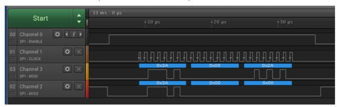
8. Wait for ADC complete Bit (Address: 0x05 / Value: 0x01)
