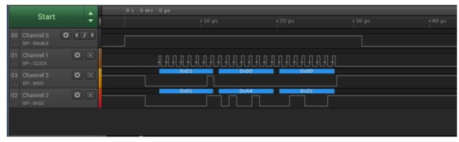
9. Perform Readout (Command: 0x90 / 5 Bytes transferred)
