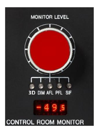
• If Lock Monitor Level is selected in the Settings screen, only the stereo (all LEDs off) and 3D monitoring options can be toggled.
