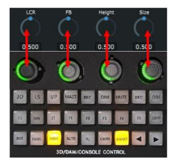
The LCR parameter is mapped to encoder 1 on the console surface. Rotating the encoder clockwise or anticlockwise will adjust the LCR coordinates, panning the selected object to the left or right of the listening position on the X-axis.
