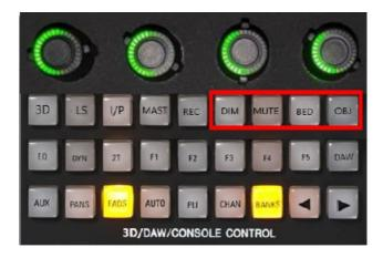
• DIM – activates the Dolby Atmos Renderer Dim control. Attenuating the renderer's output by -20dB
