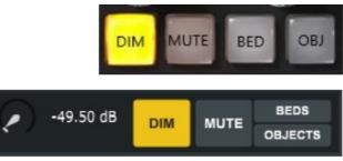
MUTE – Activates the Dolby Atmos Renderer Main Mute control. Main Mute is an output mute (post-meter) and cuts the output from the Dolby Atmos Renderer.
