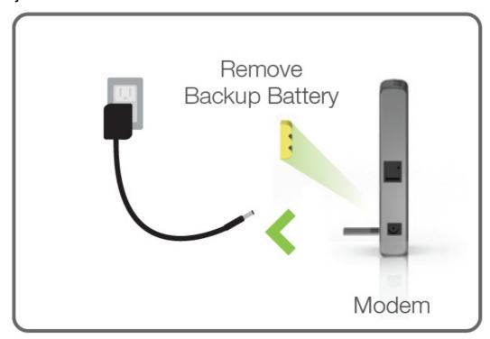
Power off the modem by disconnecting the modem's power adapter from the power outlet. If your modem has a backup battery, remove the backup battery from your modem. Do NOT power on your modem until Step 4.
