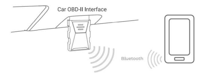
Tap Diagnostics on the home screen, then tap at the top right of the screen to establish a Bluetooth connection with the unit. When connection is established, the LED light on the unit will turn solid blue.
