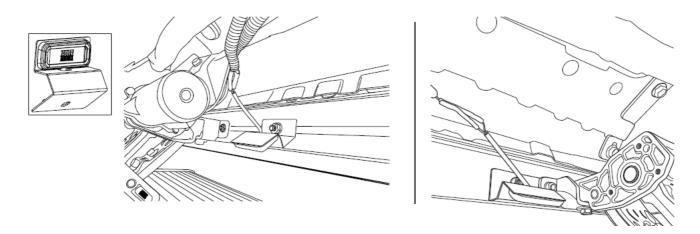
Using supplied butt connectors (19), connect the lamp wires. Red to Red, Black to Black. Once Crimped use heat gun to shrink tube. Close and wrap conduit with electrical tape. Secure all loose wires with zip ties (16). Pull lamp wires upward to avoid any wire snagging.
