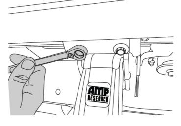
Install provided Spacer (15) and M6 Bolt (10) into upper mount as shown on both the Drive and Idler linkages. Do not tighten.
