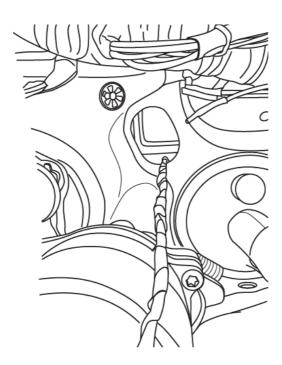
Locate the following wires and connect with supplied Posi-Tap™ (26) to the following wire colors listed below.
