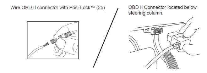
OBD II install: Use Supplied Posi-Lock™ (25) connectors to attach the Plug and Play Module to the Harness. Attach matching colors on the harness to the wires on the module. Plug in module to OBD II port on the vehicle. Secure harness with supplied tie wraps. Note: If the OBD II pass thru harness (76404-01A) was purchased see install sheet supplied in packaging. The pass through harness allows for an open port for other accessories. See below for a brief description.
