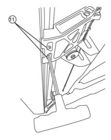
Using a 13mm socket Torque linkage bolts 4x (9) from step 5 to 16 ft-lbs. Next use a 10mm socket, torque linkage spacer bolt 2x (11) from step 6 to 8 ft-lbs. Once linkages are tight cycle board to verify steps deploy under own weight.
