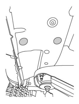
Attach bracket (27) using M10 Hex Flange Bolts (8). **Driver side shown.**
