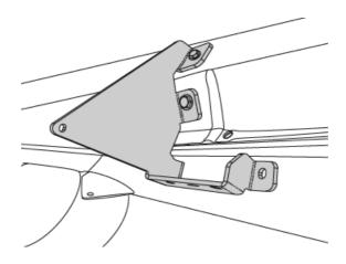
Insert 6 Carriage bolts (#12) into slot on rail (#2) from either end of rail. Add Light Bracket (#14) on the 3rd and 4th bolt. Insert Flange nut (#13) onto bracket tab to attach light brackets (14) into position shown. Dimensions shown are for reference. Leave loose to allow for adjustment.
