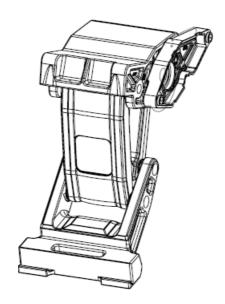
Motor Linkage assembly Passenger
