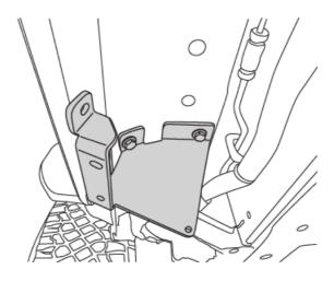
Locate Rear Drive linkage location. If plastic plugs are present remove plastic plugs to expose threads.
