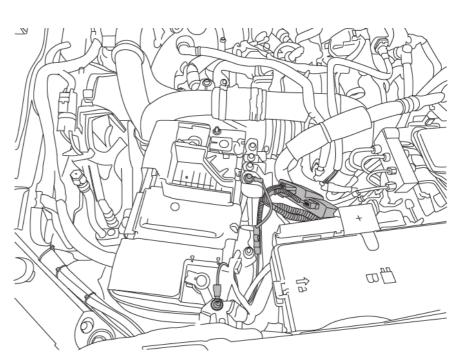
Route the two wire harness legs down over to each wheel well. Long leg will run across to passenger side, short leg will run down to driver side. Ensure loom is free from steering and exhaust components. Secure harness with Zip Ties (16).
