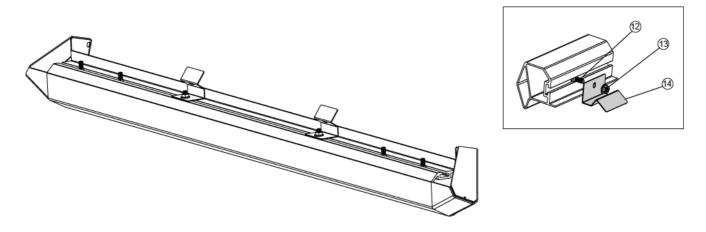
Set rail up into position, center in rocker panel area. Starting with the rear bracket, work towards the two front brackets. Insert Flange nut (13) to bolts to attach rail to brackets. Start from rear of vehicle and torque 4x M10 Flange Nuts (13) to 16 ft-lbs.
