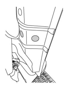
Attach bracket (28) using M10 Hex Flange Bolts (8). Driver side shown.
