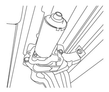
On driver side, run Wire Harness leg down and along underside of the vehicle floor and frame to rear Drive Linkage. Connect harness to motor and secure harness with tie wraps.
