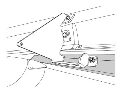
Mount front drive linkage onto rear location on driver side. Thread supplied M8 Hex bolts (#9) into front drive linkage. Repeat step for Front idler linkage. Do not tighten.
