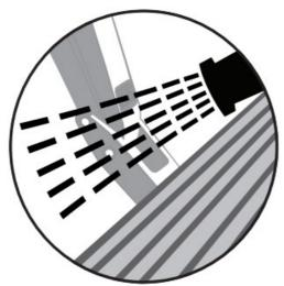
**Maintenance:** In adverse conditions, debris such as mud, dirt, and salt may become trapped in the running board mechanism, possibly leading to unwanted noise. If this occurs, manually set the running boards to the deployed position and flush the front and rear hinge arms with a high-pressure car wash wand.
