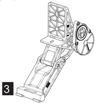
Slide the front mounting T-nut into position, place the board(1) about 5 to 6 inches from the front edge of the front door. Use fasteners(11) to attach boards, finger tighten only. Align the rear T-nut and bolt it to the rear linkage. Then tighten all 4 fasteners to 10 ft-lbs.
