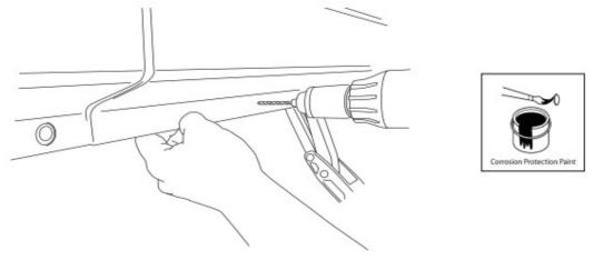
Insert grommet(17) into drilled holes.
