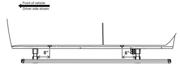
Measure down 1/2" from the top of the pinchweld. Center punch and drill a 1/8" pilot hole then drill a 19/64" hole through the pinch weld at marked locations. Deburr all holes. After drilling apply paint to holes to prevent rusting.
