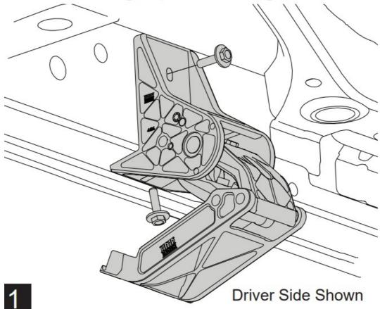
Install the Idler linkage in the First mount position at the front of the truck, for Passenger and Driver sides, using the bolts supplied (13). All plastic or rubber hole plugs need to be removed that are next to the linkage mounts. Also, an extra vertical seam-sealer bead may need to be removed from the front linkage mounting surface. Torque fasteners to 16 ft-lbs. (22 N m).
