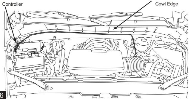
Remove the cover on the battery top box and connect the Black wire to the battery terminal accessory stud. Connect the Red wire to the stud on the positive power battery cable terminal using included Nut (18). Remove Negative terminal on battery to prevent a CEL when removing Connectors under dash in step 13. A loss of communication code may appear if battery is not disconected.
