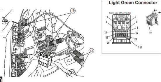
OBD II install: Use Supplied Posi Twist connectors to attach the Plug and Play Module to the Harness. Attach matching colors on the harness to the wires on the module. Plug in module (7) to OBD II port on the vehicle. Secure harness with supplied tie wraps. **Note:** If the OBD II pass thru harness (76405-01A) was purchased see install sheet supplied in packaging. The pass through harness allows for an open port for other accessories. See below for a brief description.
