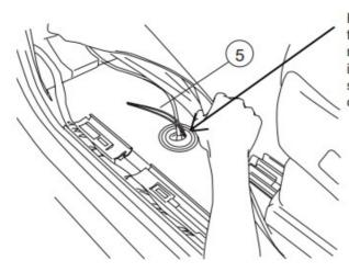
Route the two trigger wires towards the rear of the vehicle above the body mounts, and up through the hole made in the rubber grommet in the previous step. Secure harness with supplied cable ties.
