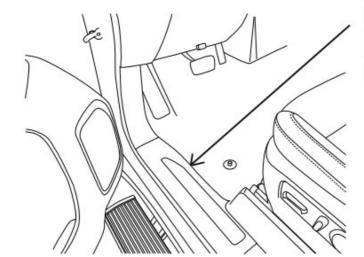
Remove the driver side door sill trim and kick panel carefully. Pull up the carpet, and poke a small screwdriver through the rubber insulation material.
