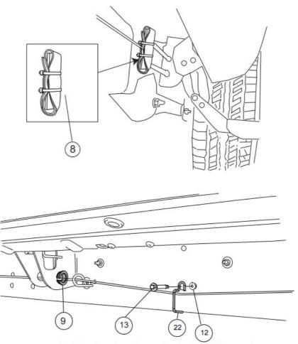
Install nut and washer on back side of frame rail
