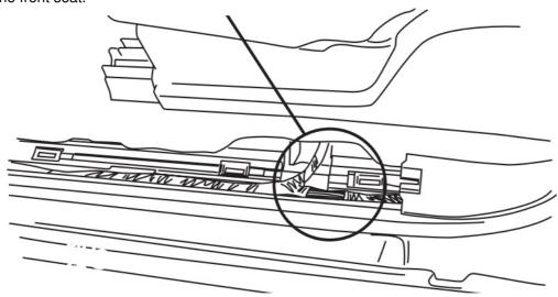
**Crew Cab Only.** Using supplied Posi-Tap<sup>™</sup> connector, splice shorter trigger wire into wire found in Step 16. Otherwise tape off short wire.
