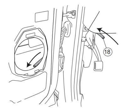
Feed longer wire of Step 13 through tube into door and pull out plastic tube on door side. Route wire along harness to switchplate.
