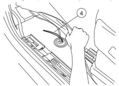
Seal holes with silicone glue and cover with tape so carpet does not stick to glue.
