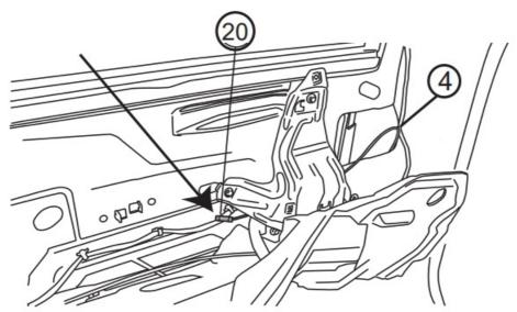
**Note:** On Hybrid models trigger wire colors will not match up because wire harness is flipped. On each side of the vehicle measure from the front edge of door line on the pinch weld to the specified lengths below. Measure at 22" for front LED Light and 65" for rear LED Light.
