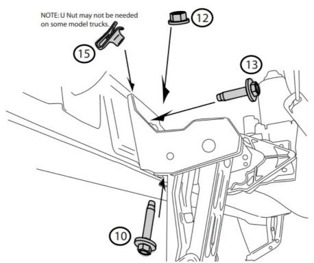
Set linkage into second to last Sheetmetal tab / hole from rear. Use supplied bolt (10) and nut(12) to hold in position. Install bolt (13) into upper mounting hole and snug both bolts. Torque upper bolt (13) to 16ft-lbs(22N m) first and then torque lower bolt (10) and nut (12) to 16 ft-lb (22N m). Repeat linkage installation on Passenger side.
