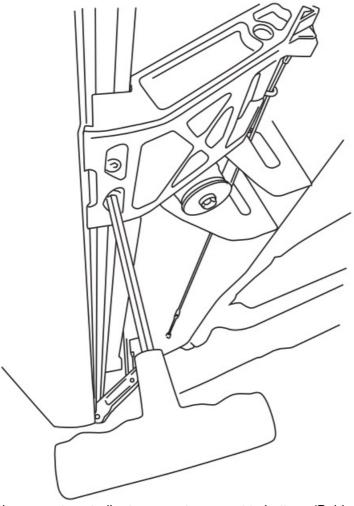
Using the two 11" cable ties, mount controller to support arm next to battery. (Behind support arm on diesel engine) On Hybrid models: Mount controller on driver's side of engine compartment.
