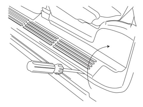
Pull up the carpet and thread both wires through the floor panel (same steps on passenger side EXCEPT drill 9/32" hole in metal and add rubber grommet). For all vehicles except Crew Cabs skip to step 18.
