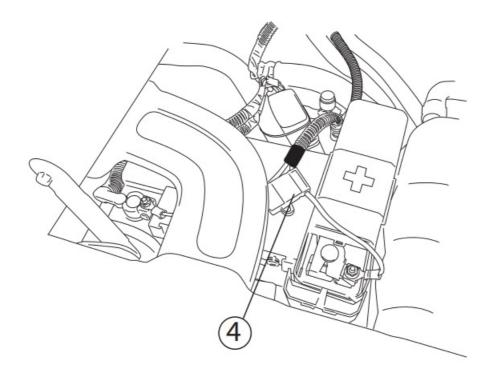
Attach ground lead to negative battery pole.
