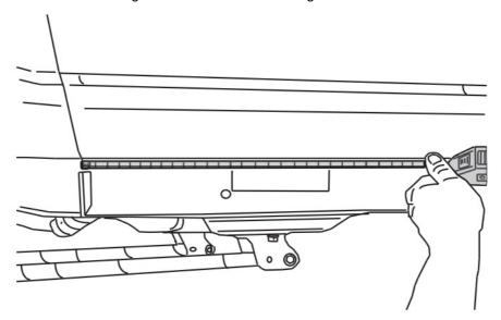
Affix lamp to rocker panel surface. Make sure the lamp is affixed to a clean, flat surface. There is a step down midway across the surface. Affix lamp just outside of step down.
