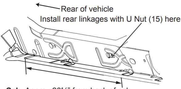
Crew Cab- Approx 261/4" from back of cab Extended Cab- Approx 11" from back of cab
