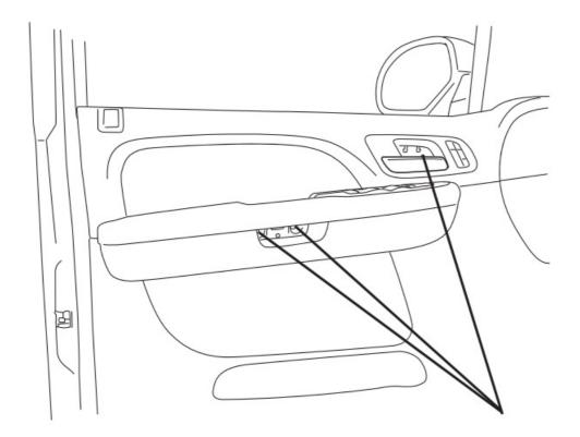
Remove door latch cable from door panel.
