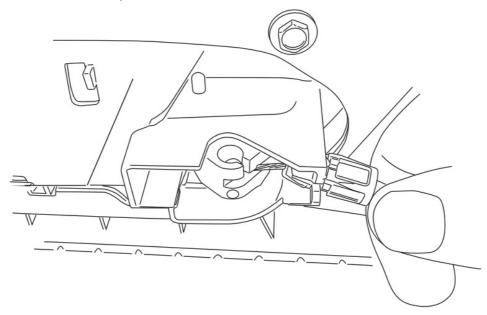
Pull back the door weather guard, unbolt speaker and unplug. Thread plastic tube through accordion.
