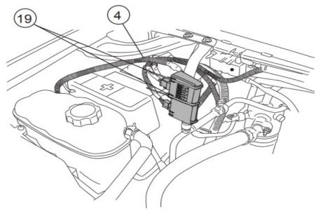
Plug in wire harness. (Ensure that locking tabs engage.)
