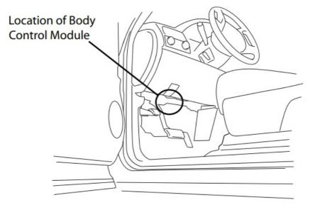
Vehicles that do not have the front door ajar signal wires in the pink connector of the BCM must have the front door panels removed in order to access the front door ajar signal wires. For these and all Hybrid models go to step 20.
