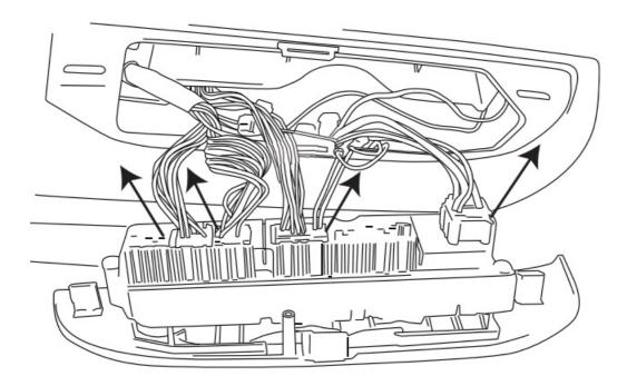
To remove door panel, first pry back tab on door lock to remove then pry off plastic covers by handle and door latch. Remove the 3 door bolts and then remove door panel by prying loose all panel fasteners.
