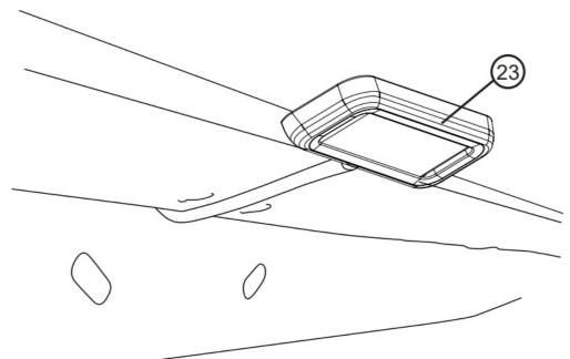
'Using supplied butt connectors, connect the lamp wires. Red to Red, Black to Black. Once Crimped use heat gun to shrink tube. Close and wrap conduit with electrical tape. Secure all loose wires with cable ties. Pull lamp wires upward to avoid any wire snagging.
