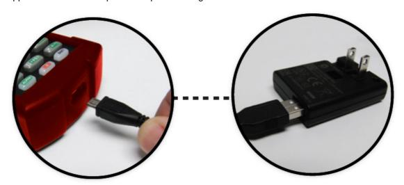
Phone chargers may or may not work properly with the LDX10 due to possible differences in charging currents. In addition, USB ports on desktop computers/laptops are also inadequate for charging and should not be used.
