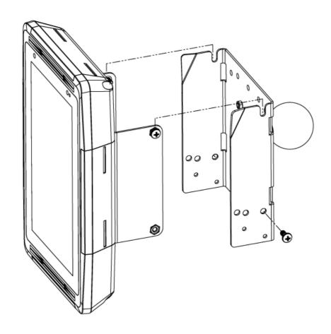
RECOMMENDED HARDWARE TO SECURE FIREBIRD VMU TO A FORKLIFT. THIS HARDWARE PROVIDES VIBRATION-DAMPENING
