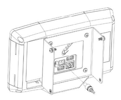
WIRE THE DC CABLE PROVIDED WITH THE CONVERTER KIT TO THE +VOUT (RED WIRE) AND -VOUT (BLACK WIRE) OF THE CONVERTER.
