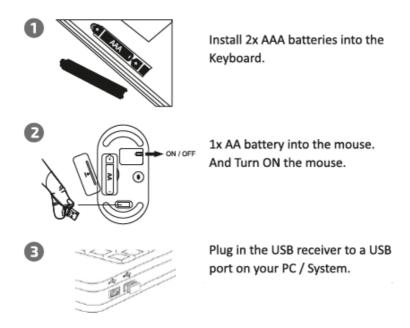
Note: USB Receiver can be found from the bottom of the Mouse
