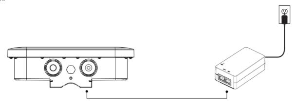
**Note:** The Access Point supports both IEEE 802.3at PoE (Power over Ethernet) or the included power adapter. You may use either one as the power source. DO NOT use both at the same time.
