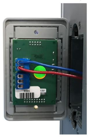
7. Connect two wires from the nurse call to the bottom terminal block in the keypad in order to operate two functions through the pillow speaker. (Optional)
