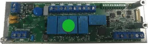
2. Connect the Master Controller input wires (Black= Line/White=Neutral) to the line voltage using silicone wire nuts.
