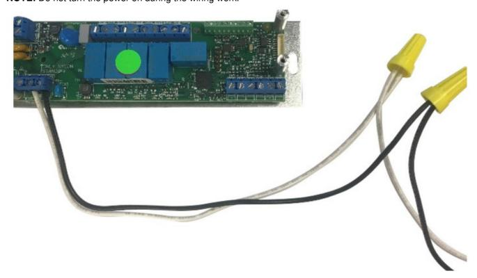
3. Connect the ground wire from the main line power to the ground wire in the fixture.
