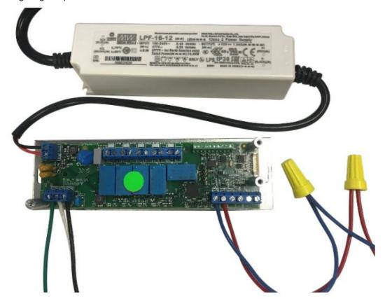
5. Connect wires for loads and dimming's as per provided wiring diagram.
