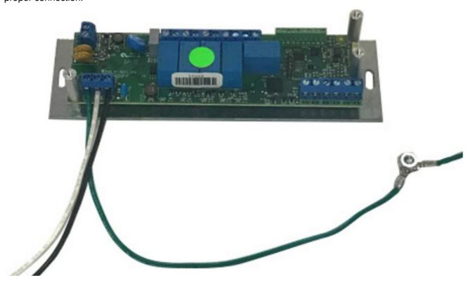
4. Connect low voltage output wires from Master Controller to the keypad using silicone wire nuts. Each keypad will connect to one Red one Blue wire provided and labeled in light fixture. Wiring should be done as per the wiring diagram provided.
