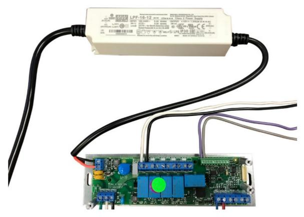
6. Connect two wires from the Master Controller low voltage output to the top terminal block on the keypad. (The bottom terminal block is used for the nurse call pillow speaker connection only).
