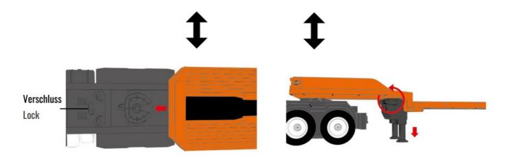
• After fitting the kingpin in the fifth wheel coupling, close the coupling using the lock.
