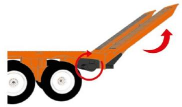
• Pull out the crank handle and turn to the left to lower the ramps. Turn to the right to raise the ramps again
