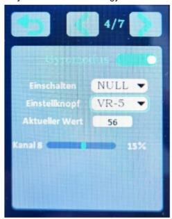
To adjust the sensitivity of the receiver, the gyro mixer of the remote control must be activated. You can choose between the VR - 5, VR - 6 potentiometer or NULL.
