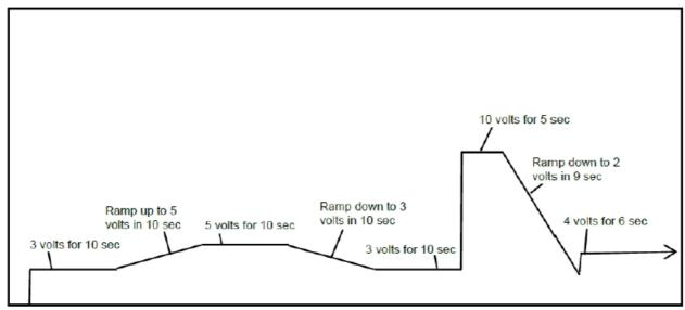
Although a single sequence is limited to 20 steps, the SUBCALL command effectively enables longer
