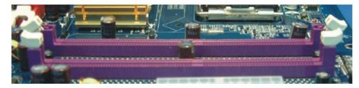
2. Align a memory on the socket such that the notch on the memory matches the break on the socket.
