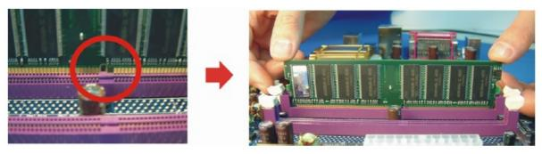
3. Lower the memory vertically into the socket and press firmly by using both thumbs until the memory snaps into place.
