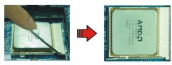
4. Smear thermal grease on top of the CPU. Lower the CPU fan onto the CPU and use the clasps on the fan to attach it to the socket. Finally, extend the power cable from the fan and insert it onto the "CPUFAN" adapter.
