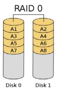
**WARNING!!** Although RAID 0 function can improve the access performance, it does not provide any fault tolerance. Hot-Plug any HDDs of the RAID 0 Disk will cause data damage or data loss.
