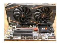
► Make sure that the gold edge connector of the graphics card is securely inserted.
