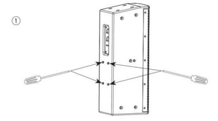
1. Unscrew four sockets on the back of loudspeaker. Do not use these removed screws for mounting – proper size screws for attaching bracket are included with RF UB55.
