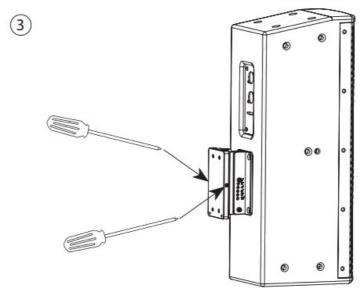
Place loudspeaker with attached bracket onto mounting plate.
