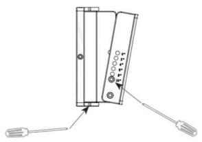
Plug audio cables and make final loudspeaker angle adjustments.
