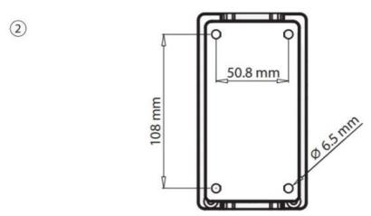
2. Attach mounting plate to the surface. Please leave required space from all sides for cables and loudspeaker angle adjustment.
