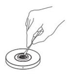
When the inner surface of the crystal glass shade or aluminum base gets dirty, the shade can be removed by turning it counterclockwise.
